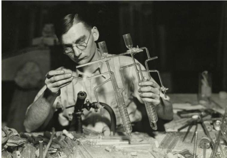
*Lewis Hine, Worker finishing the end of a sulphur determinator,
